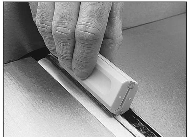
Figure 37. G3631 Jointer/Planer Knife Hone.
